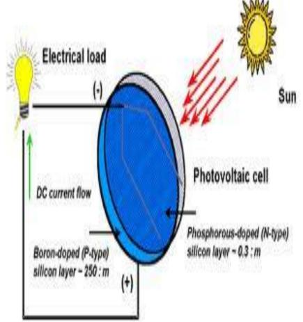
electrons and produce electricity. It contains a p type and n type semiconductors in
