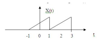
From the figure we find that T =2 and  $\Omega_0 = \frac{2\pi}{T} = \pi$ . For our convenience we take the integration interval from t = -1 to t =1. During this interval x (t) = t
