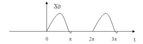
The signal x (t) =  $\begin{cases} A \sin \Omega_0 t \text{ for } 0 \le t \le \pi \\ 0 \text{ for } \pi \le t \le 2\pi \end{cases}$
