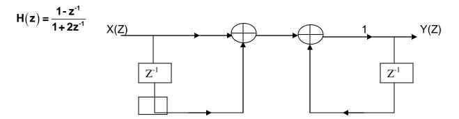
24. Draw direct form II (non-canonic) structure for transfer function [CO5-L1]
